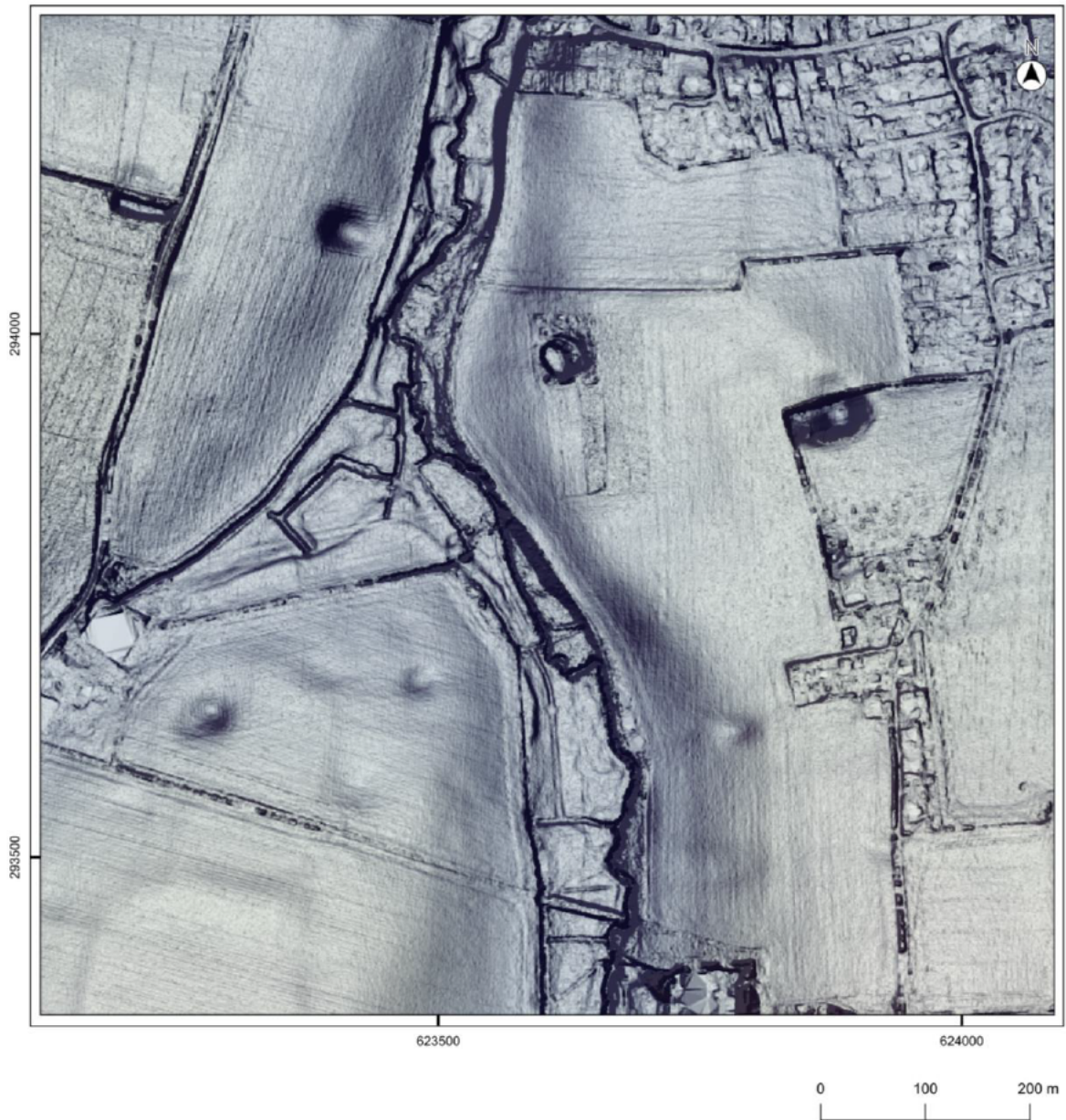
Illus 20. Unannotated LiDAR DTM imagery at 1m resolution with hillshade and colour ramp showing features HA 53 - 56
